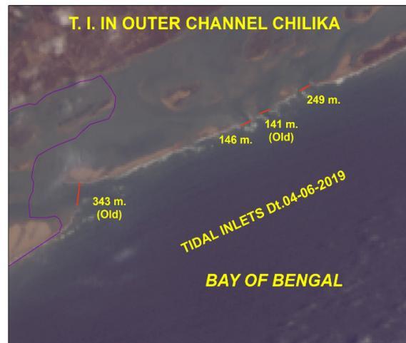
**Fig. 5** (a) The 2 TI's in Chilika before the TC Fani (dt.4.2.2019) (b) The 4 TI's in the same outer channel on 4.6.2019.
